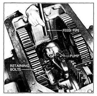
Fig 179 Fitting Hydraulic Pump Feed Pipe
