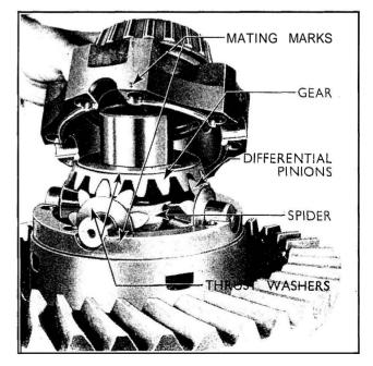
Fig. 175 Assembling Crown Wheel and Differential
