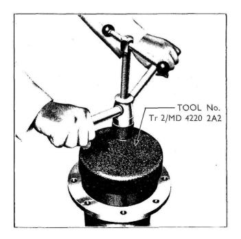
Fig. 172 Removing Axle Shaft Inner Cups
