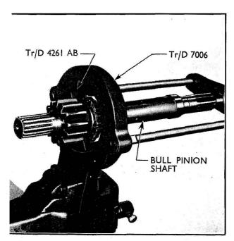
Fig. 167 Removing Bull Pinion Shaft Bearings
