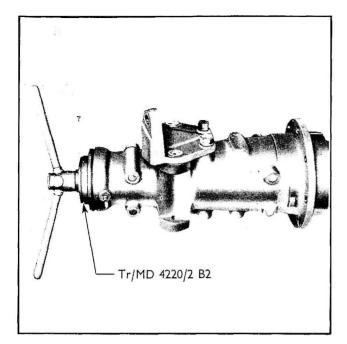
Fig. 174 Fitting the Shaft Bearing Cups
