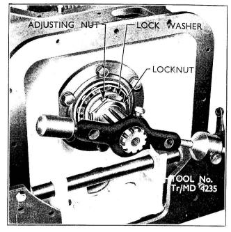
Fig. 177 Checking Drive Pinion Bearing Pre-load
