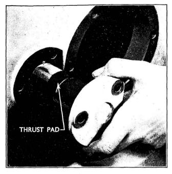
Fig. 178 Fitting the Thrust Pad
