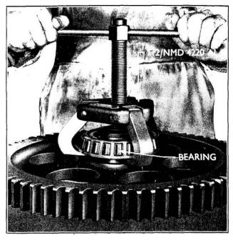
Fig. 173 Removing Large Reduction Gear Bearing
