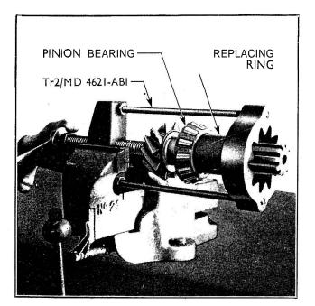
Fig. 176 Replacing Drive Pinion Bearing
