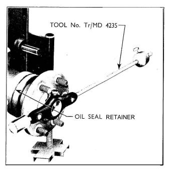
Fig 171 Checking Rear Transmission Shaft Pre-load
