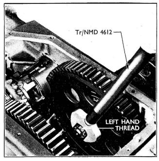
Fig. 170 Pitting the Large Reduction Gear
