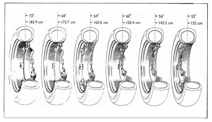
Fig. 166 Rear Wheel Width Adjustment
