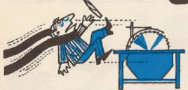
.... install or remove the belt while the belt pulley is in motion.....
