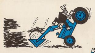
... fail to check that weight is properly distributed on the tractor....
