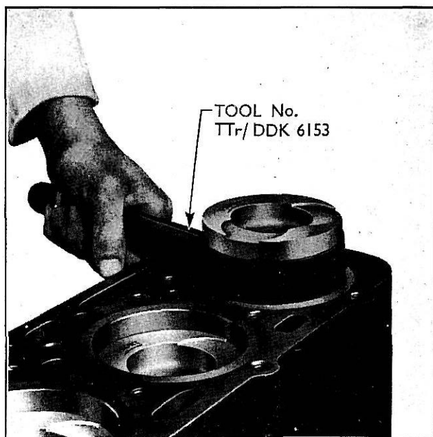
Fig. 21 Fitting Pistons
