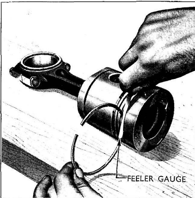
Fig. 23 Checking Ring to Groove Clearance
