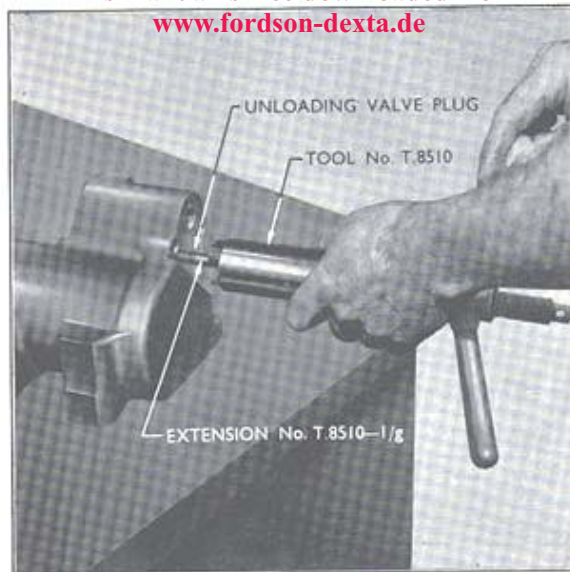
Fig. 53 Removing the Unloading Valve Plug
