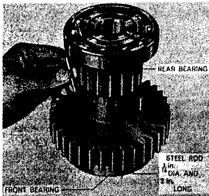
Fig. 211—Secondary countershaft front bearing can be removed by pressing against steel pins inserted through shaft against inner bearing race as shown.
